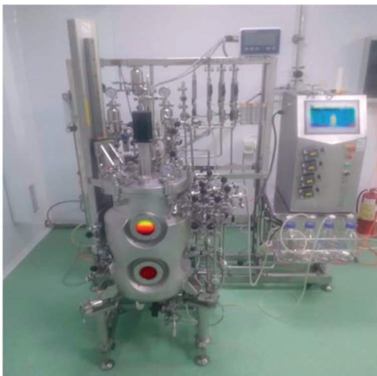
Figure 1 - Bioreactor for suspension cultivation
