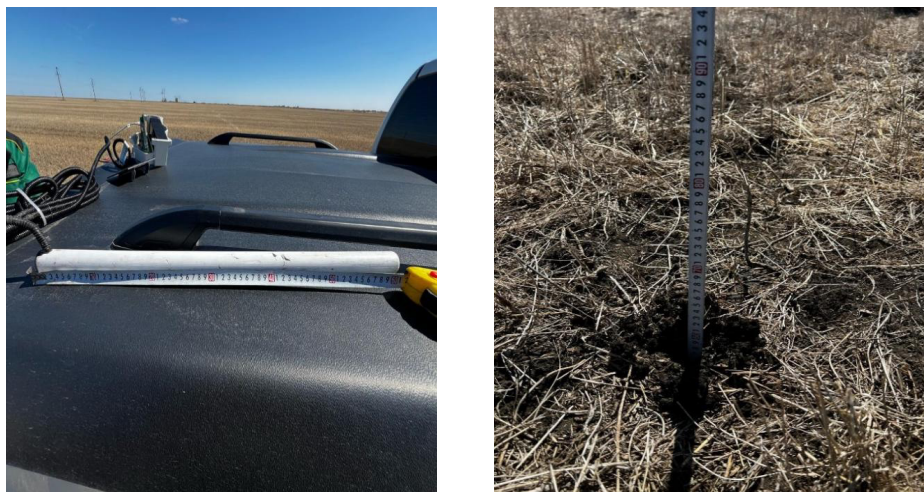
Figure 5 – Sentek Drill & Drop probe for 60 cm depth probe view and installation
