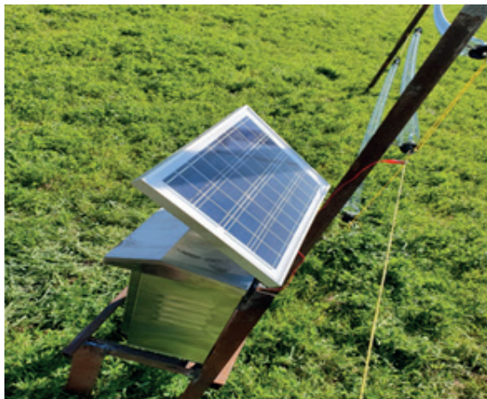
Figure 4a – Electrified fencing for livestock control
