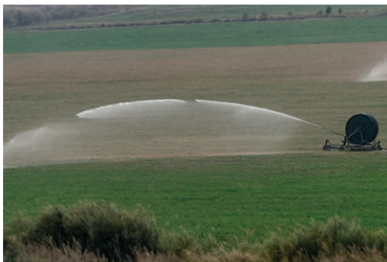
Figure 2 – Irrigation using a drum-type sprinkler machine on cultivated pastures
