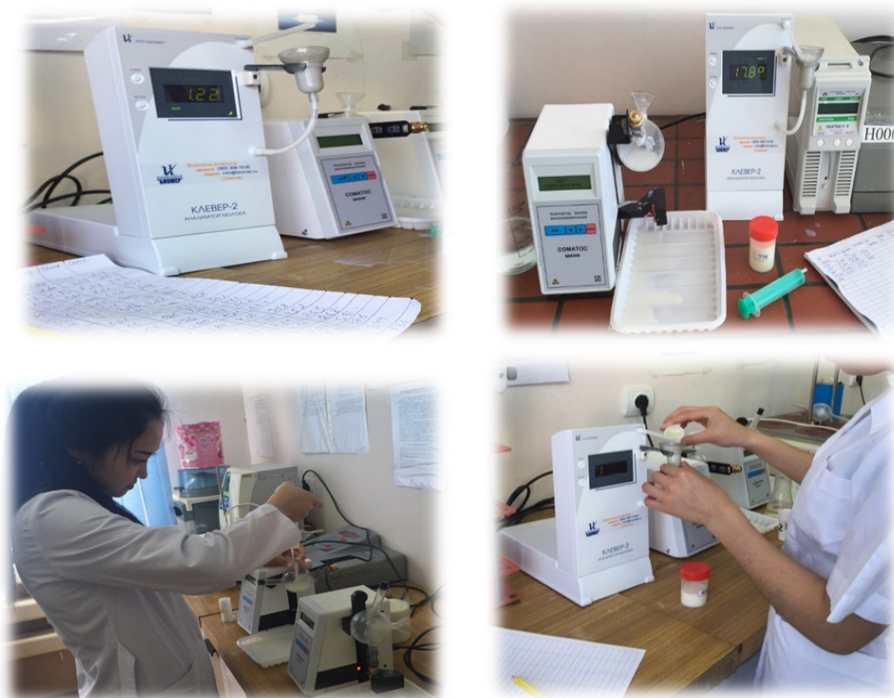
Figure 2 - The process of milk analysis on the analyzers Clever 1M", "Clever 2M", "Somatos-Mini»
