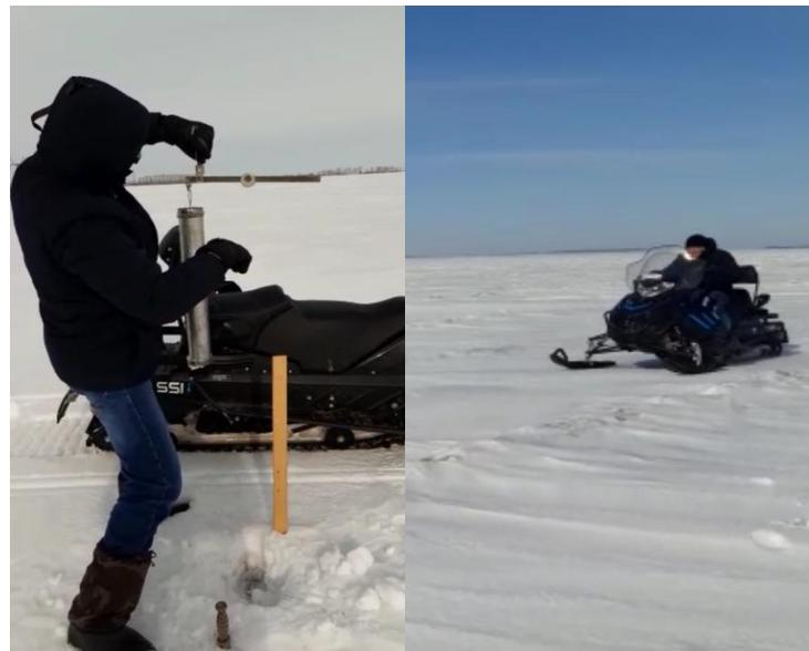
Figure 2 - Process of measuring snow height with metal ruler and density via weight snow gauge VS-43 using a snowmobile for convenient and quick movement
