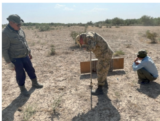
Figure 3– Selection of soil samples to determine soil moisture
