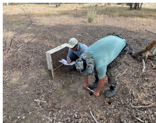
Figure 3– Selection of soil samples to determine soil moisture
