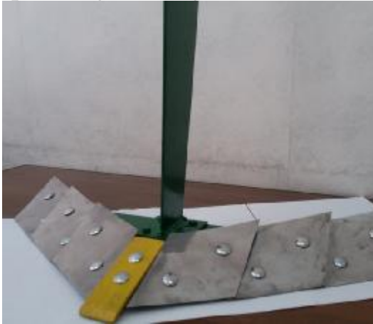
Fig. 6. The deep-cutting working elements with a variable cutting angle
