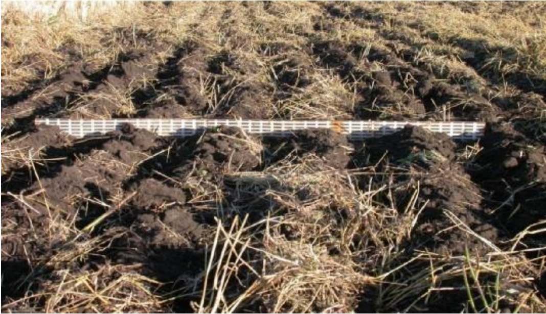
Figure 12 – Ridgeness of field surface after passing the disc header at the speed of 6.2 km / h
